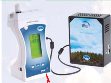
IAQ Meter (CO 2 , CO, Formaldehyde, TVOC, O 3 , PM10, Temperature & Humidity)
