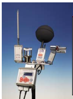
Thermal Comfort System: Temperature, R. Humidity, Mean Radiant Temperature, Airspeed, PMV, PPD calculation & Simulation.
